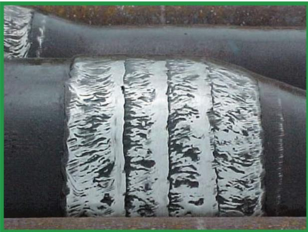
Figure 3.22.10 Tuboscope TCS 8000 on used pipe - Acceptable.
