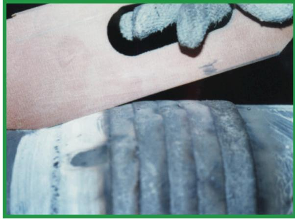
Figure 3.22.5 Weld profile at box tool joint taper - Acceptable. (Photo courtesy of Arnco)
