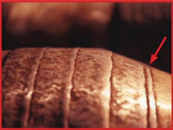
Figure 3.22.3 Improper tie-in on 18° shoulder, repaired with single weld - Unacceptable. (Photo courtesy of Arnco)
