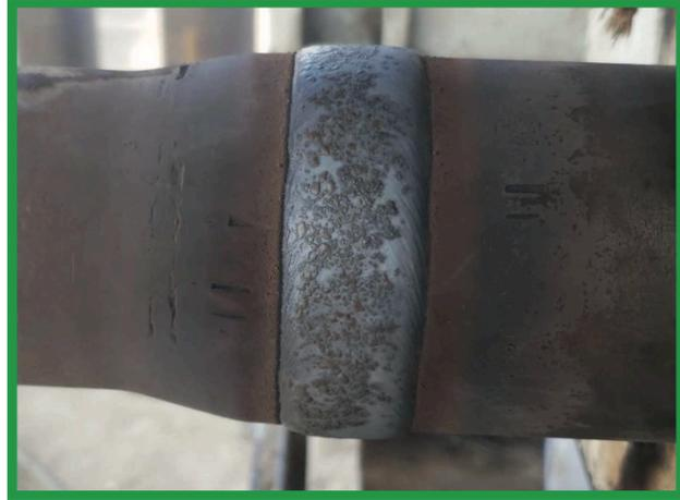
Figure 3.22.15 Hardbanding (350XT) applied to a workstring tubing connection - Acceptable. (Photo courtesy of Arnco)
