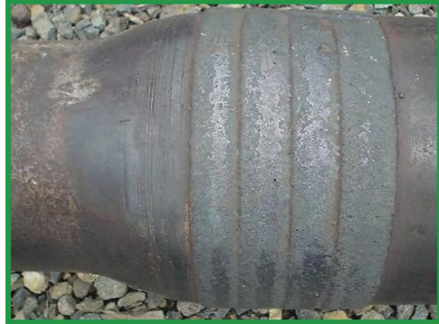
Figure 3.22.9 Tuboscope TCS Titanium on used pipe - Acceptable.
