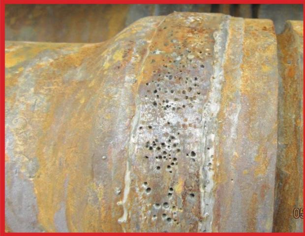
Figure 3.22.14 MStar on used pipe with excessive porosity Unacceptable. (Photo courtesy of Liquidmetal Coatings)
