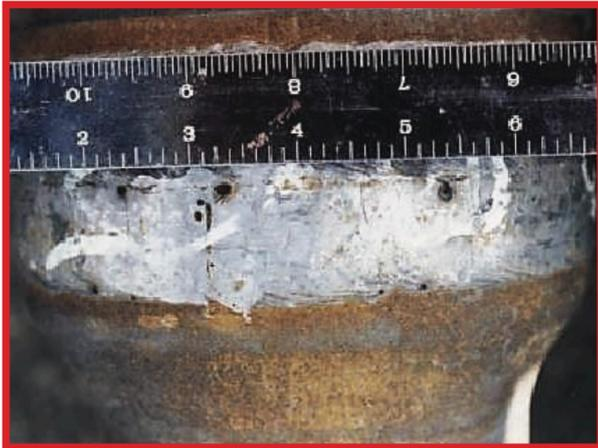
Figure 3.22.1 Voids and holes > 1/16" - Unacceptable. (Photo courtesy of Arnco)
