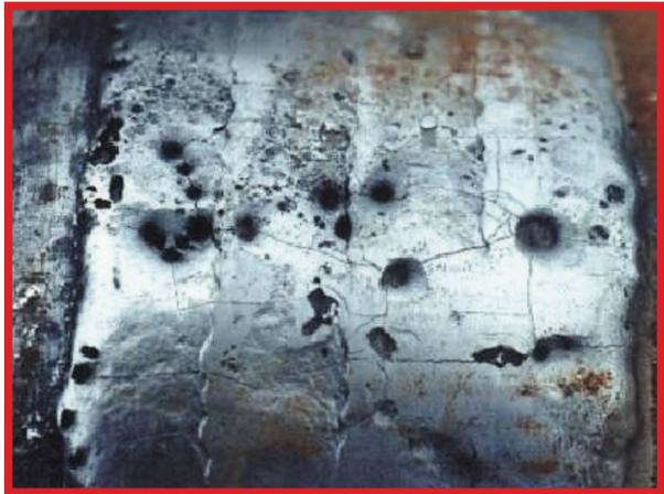
Figure 3.22.7 Excessive porosity in worn layer - Unacceptable. (Photo courtesy of Arnco)
