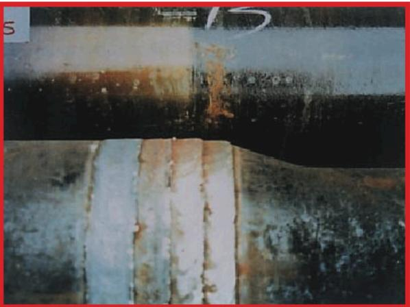
Figure 3.22.6 "Stair-stepped" weld bead profile and not flush on 18° shoulder - Unacceptable. (Photo courtesy of Arnco)
