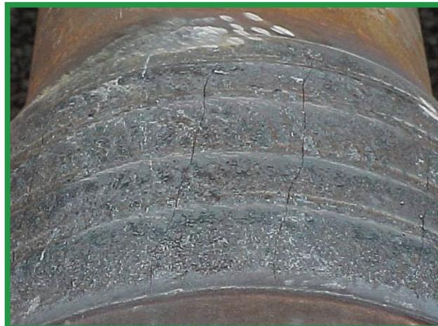
Figure 3.22.11 Tungsten Carbide cracks - Acceptable.
