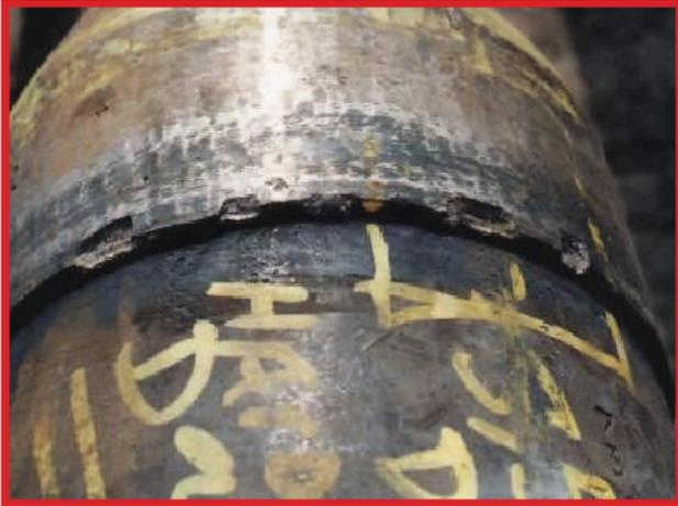
Figure 3.22.8 Flaking or chipping - Unacceptable.
