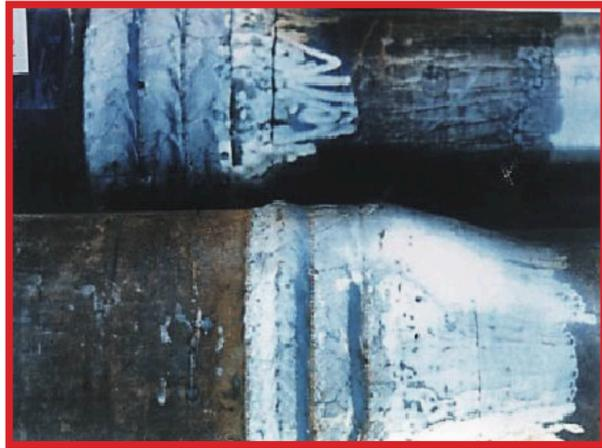
Figure 3.22.2 Weld bead profile "humper" in middle of weld bead - Unacceptable. (Photo courtesy of Arnco)
